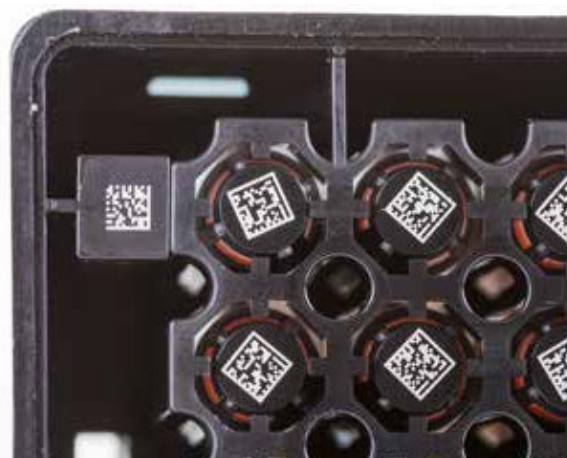
2D orientation coded rack base allows automatic detection of orientation by instrumentation
